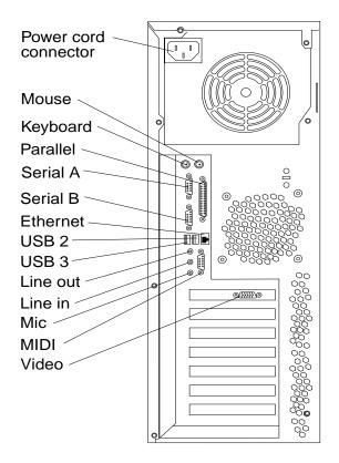
**Note:** If the server is a SCSI model, the SCSI adapter will be located in PCI slot 1; the external connector will appear in the slot below the video connector. See "System and PCI extender board options connectors" on page 35 for the location of the PCI slots.
